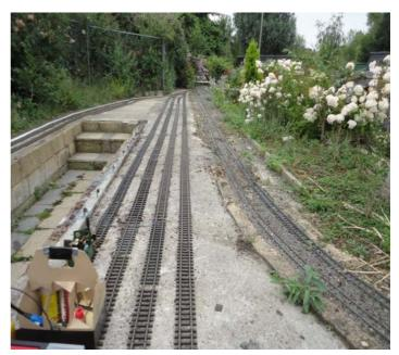
The gauge of this railway is 45mm and this allows the running of many different scale rolling stock. The picture on the left shows a 16mm/ft gas fired steam locomotive which is gauge adjustable, that is 45mm and 32mm. Not radio controlled so is free running, not too fast so the operator can get to the engine if need be.
